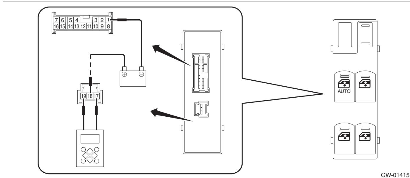
3) Operate the switch - power window main and check the output.
